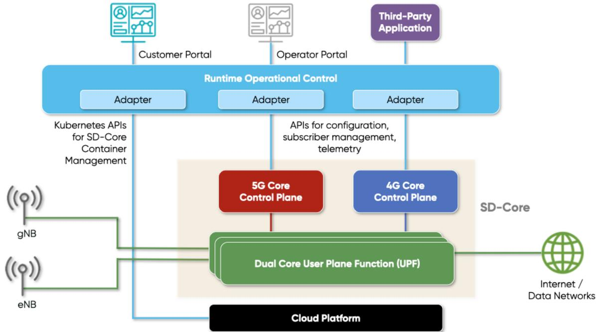
SD-Core leverages control plane components of the Free5GC project and the ONF OMEC project, building on both of these upstream open source projects by adding cloud native capabilities for scaling, resiliency and multi-cloud agility. It also includes three separate User Plane Function (UPF) implementations, and all of which are designed to be deployed throughout the edge of the network with each optimized for specific use cases:
